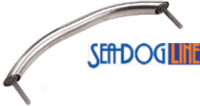
Sea Dog Stainless Steel Grab Rails Formed 304 Stainless 3/4" O.D. tubing. 5/16" Stud on each end for mounting. Protrudes 2" from bulkhead.
