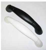
Whitecap Safety Grab Handle Molded of high impact plastic, this rugged handle has a soft leather grained vinyl covering for a comfortable, no slip grip which won't corrode or discolor in harsh marine environments. Handle measures 9-1/4" long with a 6-3/4" bridge length and a 1-5/8" finger clearance.
