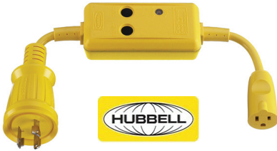
Hubbell 30A Male to 15A Female GFCI Adapter Permits use of 15A straight blade plug with 30A 125V Twist-Lock receptacle; with GFCI protection.
